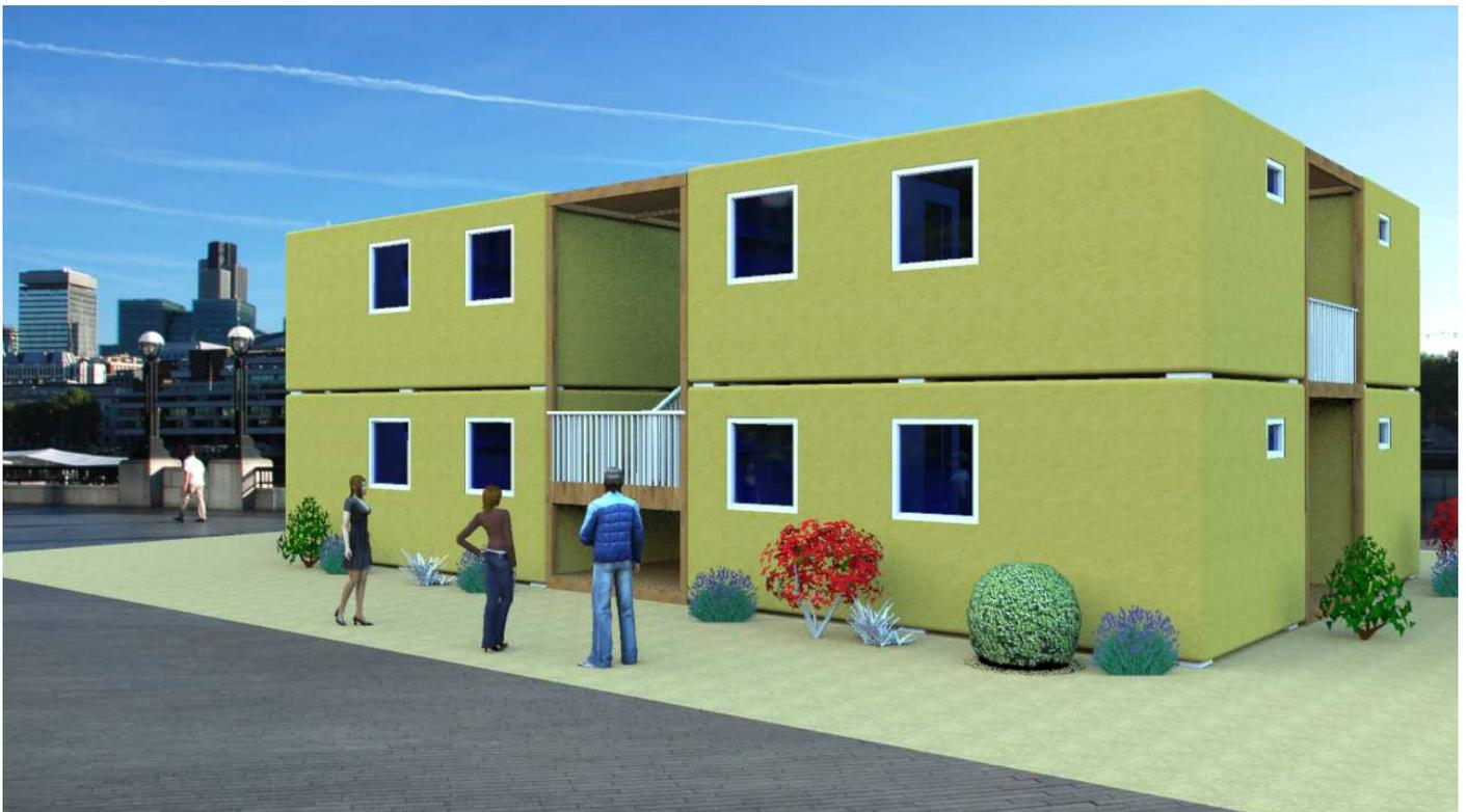
A typical stack of 8 no. compact housing units with communal walkways forming a crucifix. Each of these units is 6 m x 3m externally and has a bedroom, shower room and kitchen/living room .
